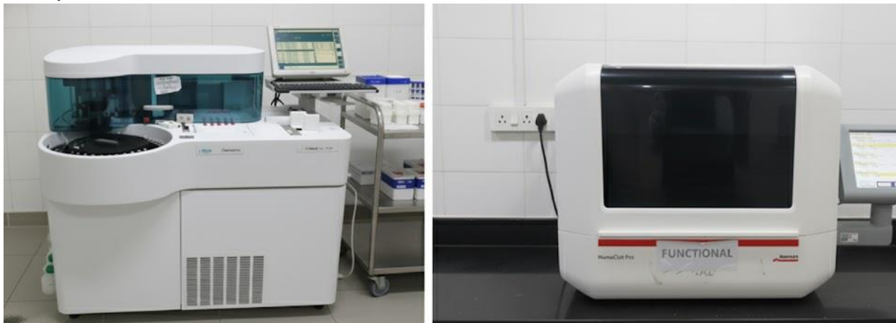
Figure 1. HumaClot Pro coagulation analyzer (Human Diagnostics) used in this study to quantify D-dimer from 3.2% sodium-citrate plasma via immunoturbidimetry ( \approx 400 nm), Allama Iqbal Teaching Hospital, Dera Ghazi Khan.
