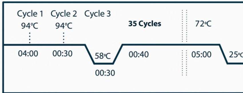
**Figure 1 Thermal Cycling Protocol**
